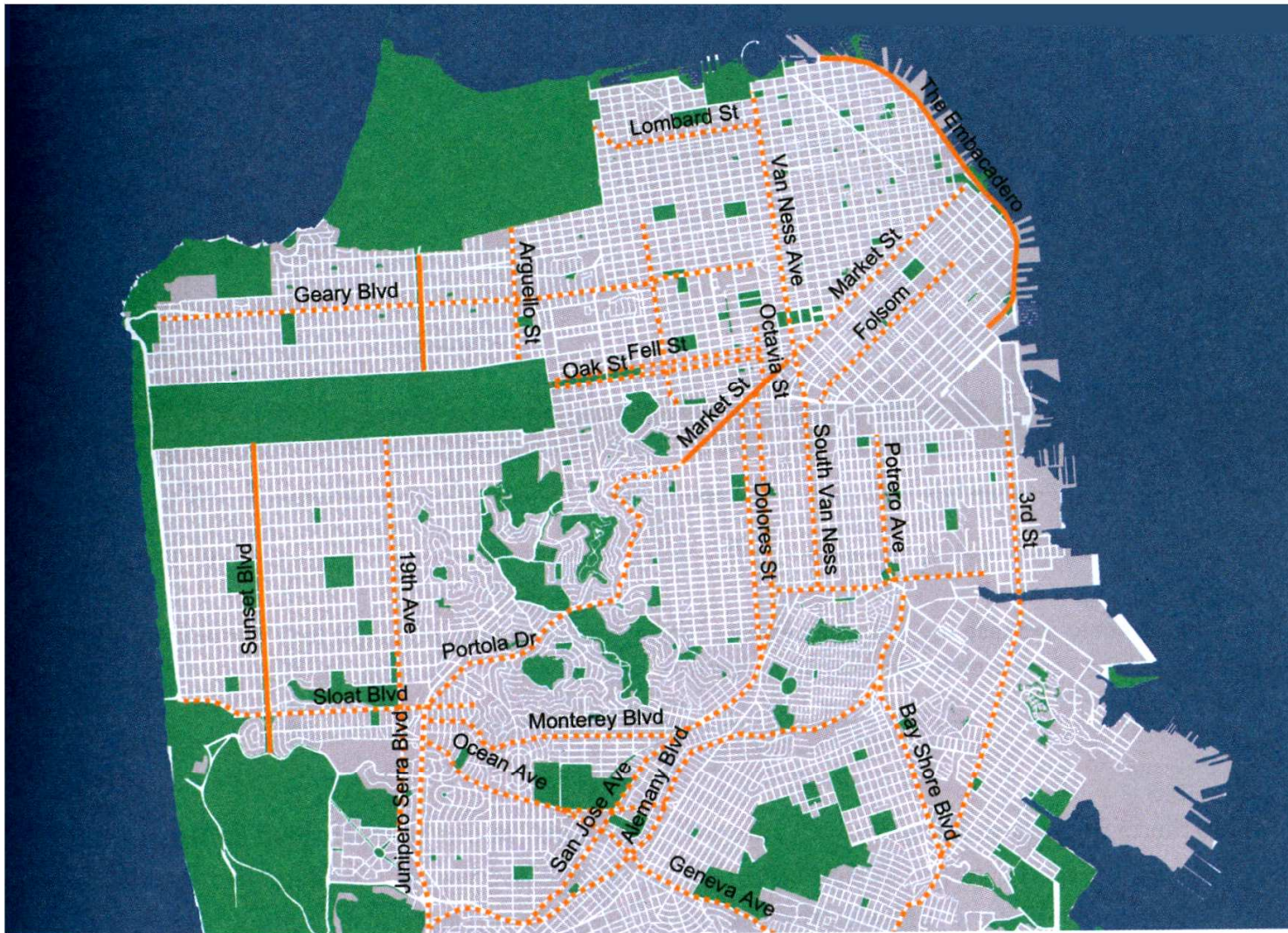
Figure 5.14 Map shows the potential for multilane boulevards citywide. Frequently configured as precursors to urban freeways, high-capacity roadways were laid out prior to World War II in San Francisco to accommodate growing commuter traffic. With the subsequent freeway building these roads are designed for access capacity. They can now be redesigned to improve the quality of life for residents that live alongside such roads. This is best done by including local access roads for residents, bike lanes, and wider sidewalks that are lined with trees.
